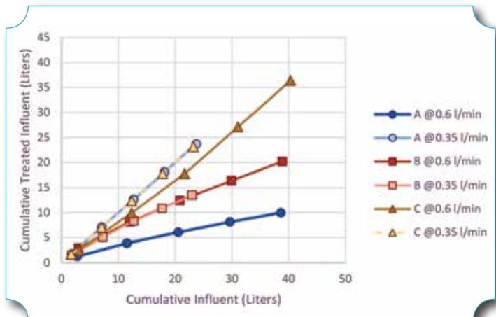
Proportion of influent treated under differing flow rates for each PSM blend.
