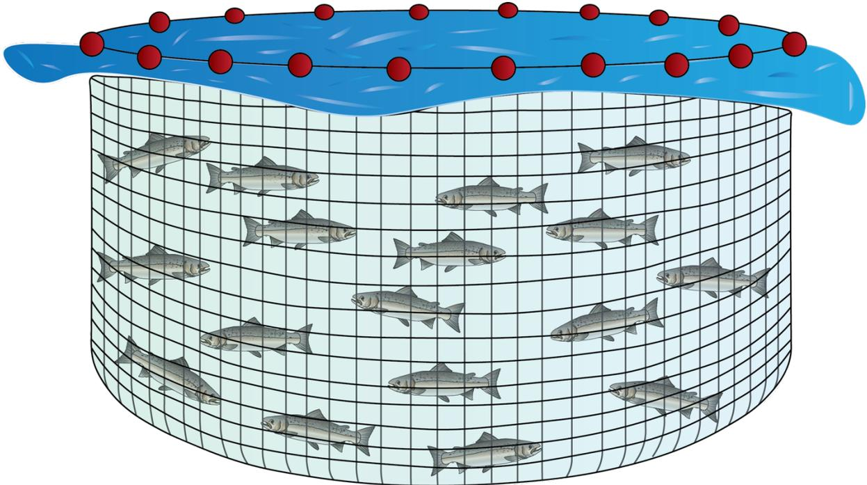
Figure 11. Close up view of one type of net pen system, where the fish are confined within a larger body of water. There are many different structures and models that can be used for coastal aquaculture operations. This is just one example of a common form.
