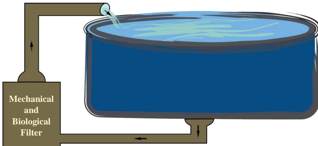
Figure 6. Example of recirculating system, which recycles its water by passing it through a series of biological, mechanical and sometimes chemical filters to remove waste and excess nutrients.
